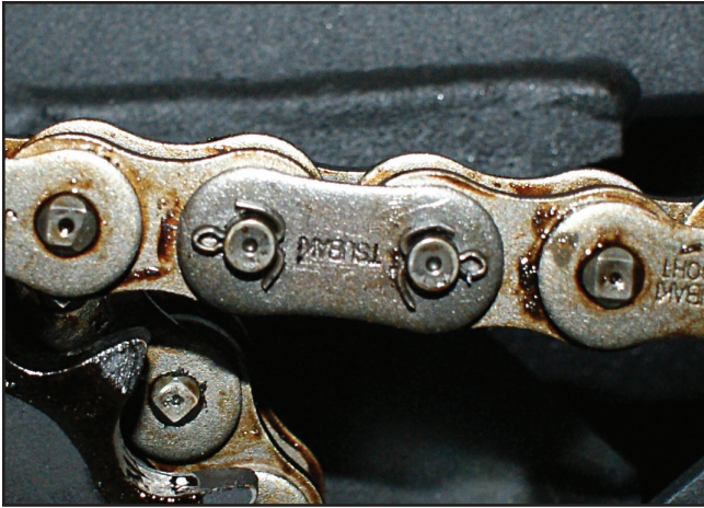
Figure 7-5. Chain connection link components.
