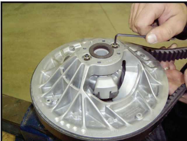
Figure 7-2b. Turn the adjustment set screw.
